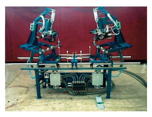
This semi-automatic machine is suitable for the processing of limited number of glasses per day; backlights are to be the classic type with one terminal tab per side.
