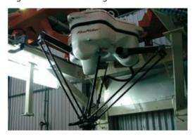
The location of the profile position by the vision system avoids the problems due to the fact that the piece is not squared mechanically under the station.
